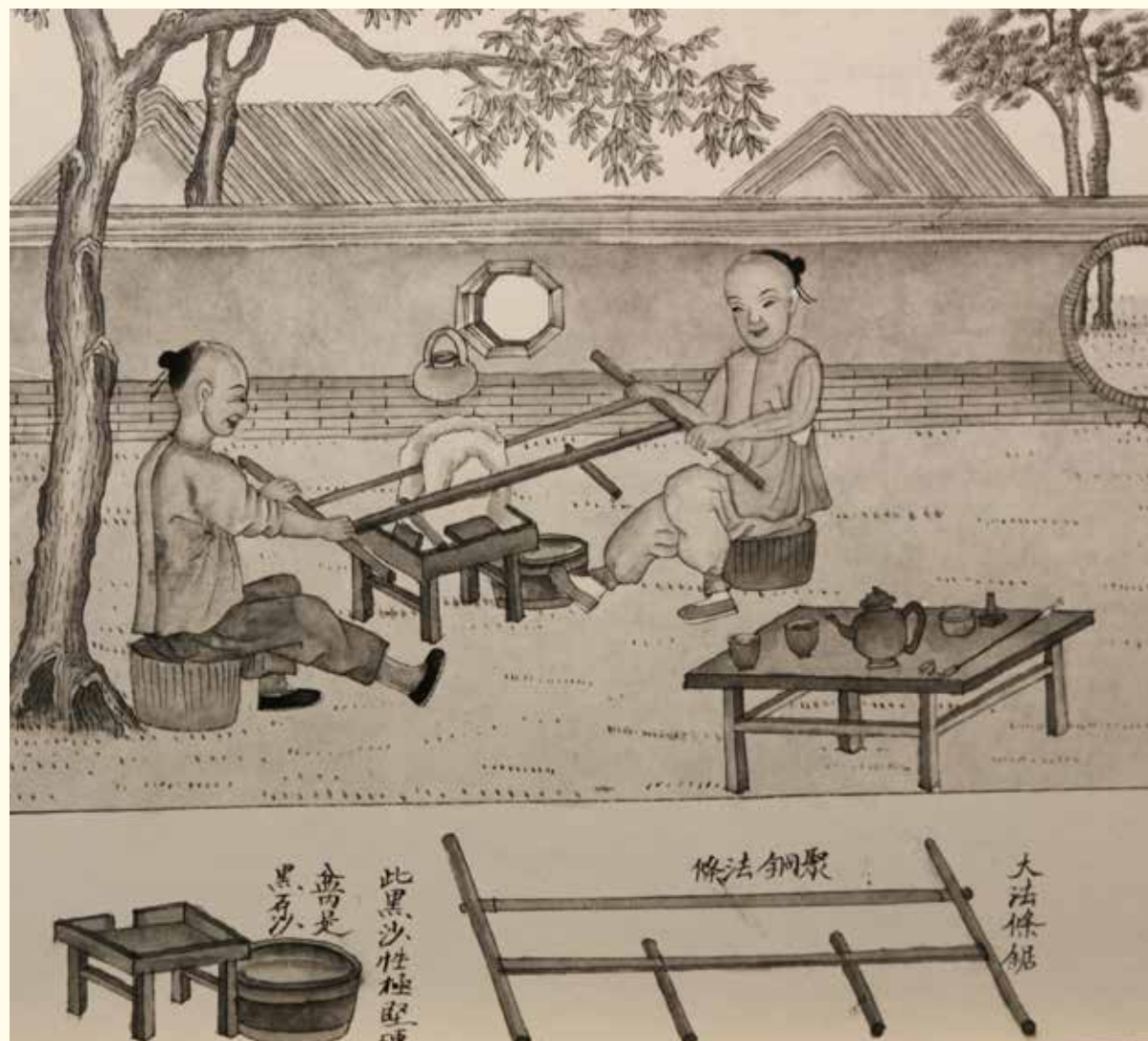
Two-handed steel saw; a pot of sands mixed with water was hung from a tree. Illustration from The Bishop Collection: Investigations and Studies in Jade (1906).
